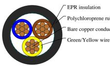
Polychloroprene rubber outer jacket Bare copper conductor
